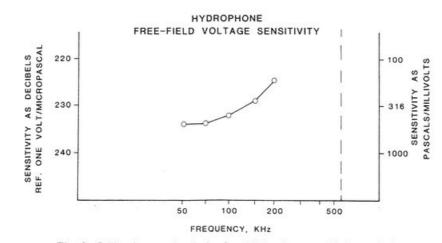
Fig. 2. Calibration graph of the free-field voltage sensitivity typical of the implanted hydrophone transducers. Reference device was a Navy Type E-27 hydrophone obtained from the Underwater Sound Reference Division, Naval Research Laboratory, Orlando, FL.
